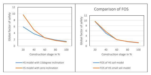
Figure 5: HS model with different inclination
