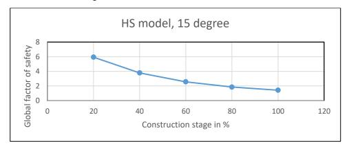
Figure 4: FOS with construction stages
