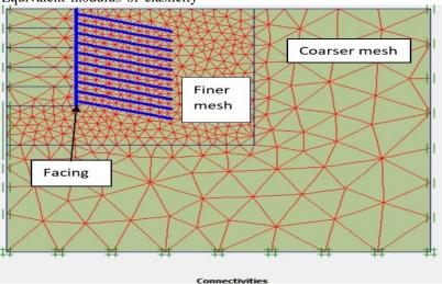
Figure 3: Simulated soil nail wall with different clustered mesh generation
