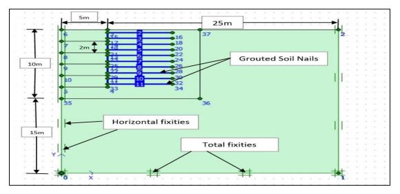
Figure 1: FEM soil nail wall with no inclination, 10m high
