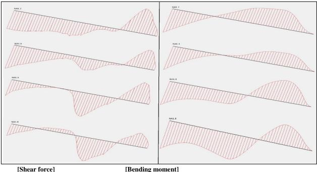
[Bending moment] Figure 8: Variable SF and BM along nail length
